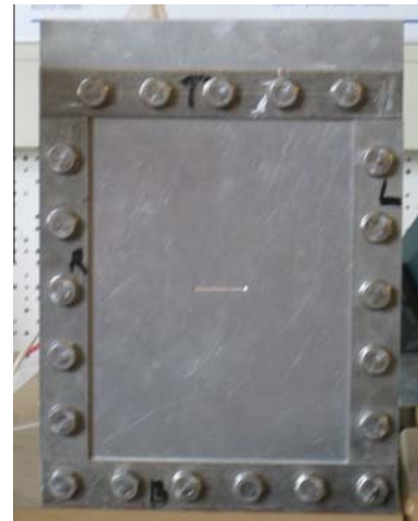
Fig. 2. Crack on the flexible plate.
