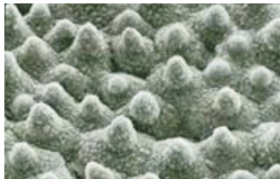
Fig. 2 A microscopic SEM image of a lotus leaf showing the two-scale roughness. (Picture adapted from ref. 7 with kind permission of Springer Science and Business Media.)
