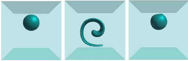
Fig. 2. Computed bubble shapes for the advection test: (left) initial bubble shape at t = 0.0 s, (centre) bubble shape at the end of the forward integration in time at t = 1.0 s and (right) bubble shape at the end of the backward integration in time at t = 0.0 s.
