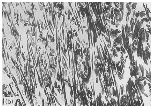
Figure 16 LM micrographs of the morphology of G-DSC samples crosslinked using pre-strain conditions cut either transverse (a) or parallel to the pre-strain direction. Magnification 10x.
