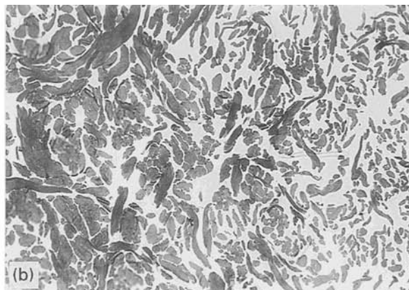
Figure 15 LM micrographs of the morphology of pre-strained N-DSC control samples cut either transverse (a) or parallel to the pre-strain direction. Magnification 10x.
