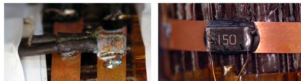
Fig. 3. Photograph of the thermal anchoring method used for the thermometer in a soldered casing and thermal paste (left) and the quench heater with alumina loaded epoxy (right).
