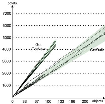
Fig. 7. Measured SNMP bandwidth consumption
