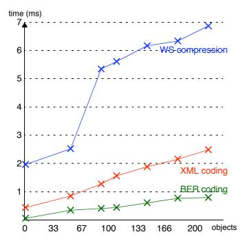
Fig. 13. CPU time for coding and compression
