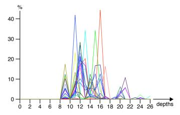
Fig. 4. SNMP OID length distribution (OID<sub>length</sub>)
