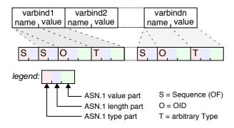
Fig. 3. SNMP variable binding list - BER encoding
