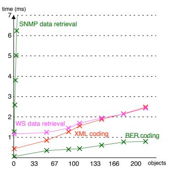
Fig. 14. CPU time for coding and data retrieval
