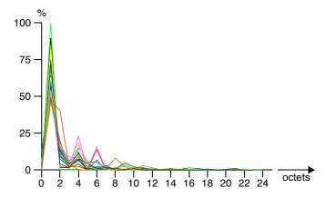
Fig. 5. SNMP object value size distribution ( $S_{ObjectValue}$ )
