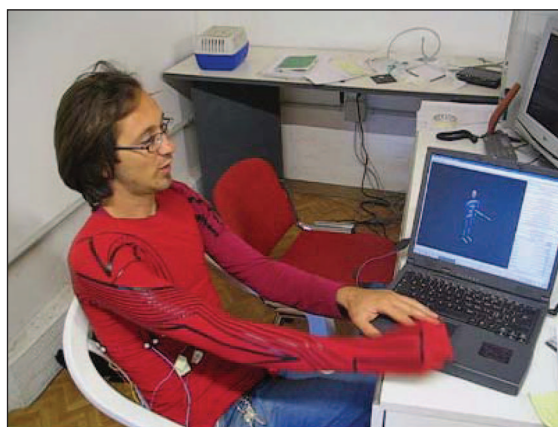
Fig. 5. A subject wearing a fabric-based upper-limb monitoring device developed for poststroke telerehabilitation is shown. The system drives a kinesthetic avatar on the laptop screen. Black stripes are both screen printed piezoresistive rubber sensors and sensors tracks (36). (Courtesy of the University of Pisa.)
