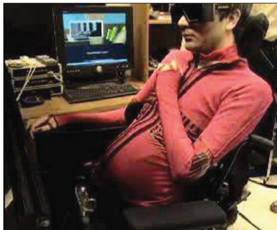
Fig. 7. A prototype of fabric-based motion classification garments based on redundant sensors arrays is shown monitoring torso and neck movement as a human-machine interface for wheelchair control (42). (Courtesy of the University of Pisa.)
