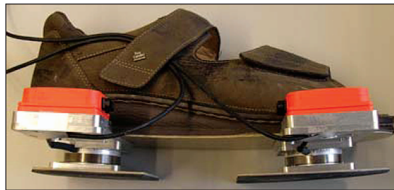
Fig. 2. Experimental instrumented shoe with six degrees of freedom force and moment sensors under heel and forefoot coupled to inertial movement sensors [24].
