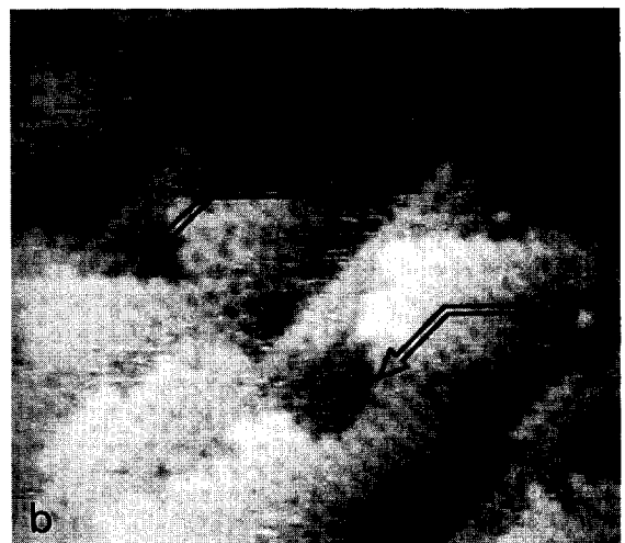
Fig. 6. (a, b) Examples of the nonbonded SB step with an effective direction of the step edge oriented at 45^\circ with respect to the dimer rows. The arrows point to the relevant edges. (a) Image of 200 \times 200 \text{ \AA} , \theta = 1^\circ . (b) Image of 260 \times 260 \text{ \AA} , \theta = 2^\circ .
