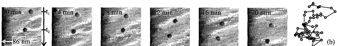
Fig. 4. Relative motion of two vacancy islands of about same size; U_i = -0.49 V, I_i = 9.5 nA. (b) Relative displacement for all 56 images of the movie enlarged by a factor of 4; \Delta t = 30 s.
