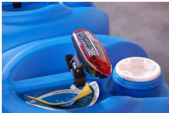
Figure 9. Wireless sensor node used for an industrial safety application [61].
