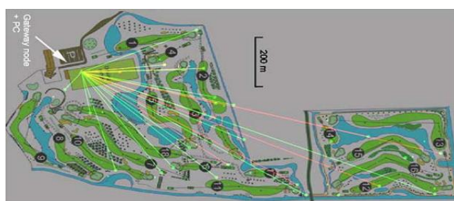
Figure 5. Wireless sensor network used for monitoring soil moisture of a golf course [41].
