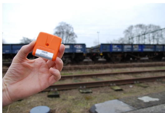
Figure 1. Smart Point: sensor node of Ambient Systems [8].
