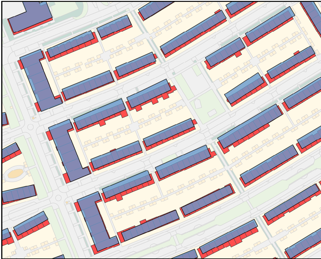
Figure 3: Large-scale building objects (in red) overlaid with medium-scale buildings blocks (in blue). The background is the large-scale dataset in dimmed colors.
