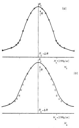
Figure 5 (a) Example of an experimental calibration curve (full curve) which fits to theory (open circles) over the entire range. (b) Example of an experimental calibration curve (full curve) which cannot be fitted to theory (open circles) over the entire range. In this case curves were fitted to overlap at least in the region of small fields but a slightly better fit can be obtained if the total field region is considered.
