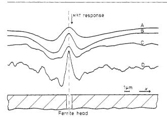
Figure 12 MRT response on the perpendicular field component of a tri-rail head  $(2g=1\cdot10~\mu\text{m})$  for: A, separation  $h=2\cdot0~\mu\text{m}$ , head current = 12 mA; B,  $h=1\cdot25~\mu\text{m}$ , head current = 12 mA; C,  $h=0\cdot5~\mu\text{m}$ , head current = 7 mA; D,  $h\simeq0\cdot05~\mu\text{m}$ , head current = 7 mA.
