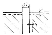
**Figure 10** Cross section of a recording head with dead layer of thickness  $l_1$  on the surface of the ferrite body and thickness  $l_2$  in the gap.
