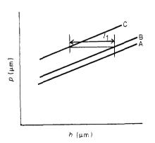
**Figure 9** Adopting the model with dead layers  $l_1$  and  $l_2$  (figure 10), it is possible to fit the computed and measured p-values. A, computed values for gap length 2g; B, computed values for gap length  $2g + 2l_2$ ; C, measured values (optical gap length 2g).
