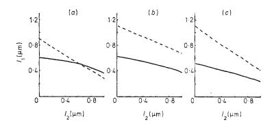
Figure 11 Relation between the values of the 'dead layers'  $l_1$  and  $l_2$  to fit the computed p to h curves to the experimental ones (— perpendicular, — tangential field component). (a) Audio head  $(2g=1.85 \ \mu\text{m})$ ; (b) type 3330 disc slider head  $(2g=2.10 \ \mu\text{m})$ ; (c) same type  $(2g=2.80 \ \mu\text{m})$ .
