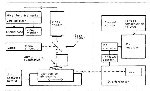
Figure 1 Scheme of the measurement system.
