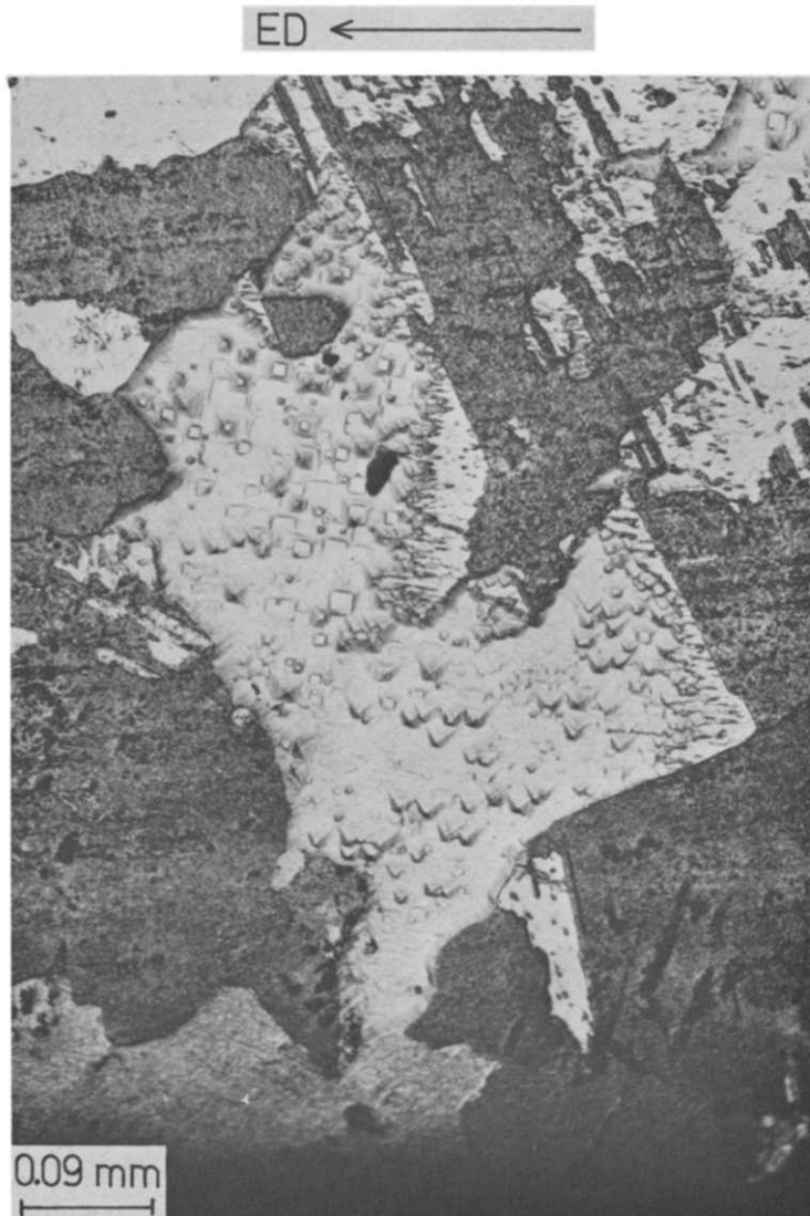
Fig. 13. Optical micrograph of the (\bar{1}10)[001] specimen, plane-strained 80.9% and annealed 60 min at 150^\circ\text{C} . The viewing plane is the constrained plane (ED-ND plane). Fraction recrystallized: 93%.
