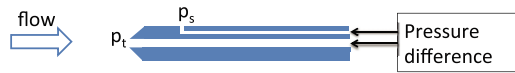
Figure 5. A schematic illustrating the measurement principle of a Pitot tube. The diameter of the tube is typically of order mm.
