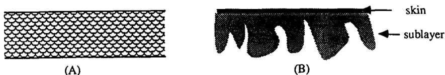
Figure 1. Schematic representation of an isotropic (A) and an anisotropic (B) membrane structure.
