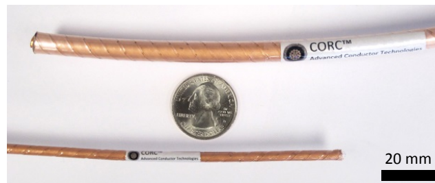
20 21 22 23 24 25 26 27 28 29 30 Figure 1 – 7 mm diameter CORC ® cable (above) made out of 4 mm wide REBCO tapes with 50 \mu\text{m} thick substrates compared to a 31 3.6 mm diameter CORC ® wire (below) made up of 2 mm wide tapes with 30 \mu\text{m} thick substrates.
