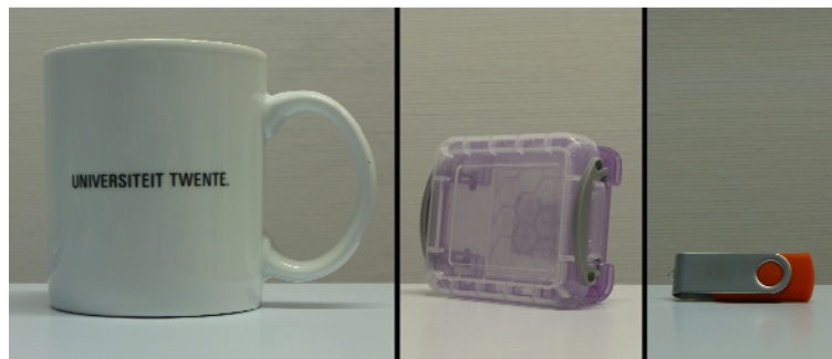
Figure 6. Three objects used in the grasping experiments. From left to right: mug (82 mm diameter), box (30 mm thickness), and USB flash drive (8 mm thickness)
