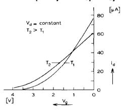
Fig 7 Generalized  $I_d - V_g$  curve of a MOSFET or ISFET as function of temperature
