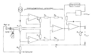
Fig 10 Principle diagram of an ISFET amplifier with additional circuitry for temperature measurement and compensation
