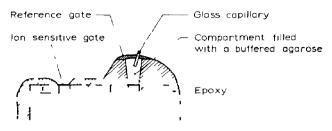
Fig 9 Construction of differential pair of a pH ISFET and a reference ISFET (after Janata and Huber [10])
