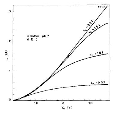
Fig 4  $I_d - V_g$  curves of a pH ISFET (after Moss *et al* [2])
