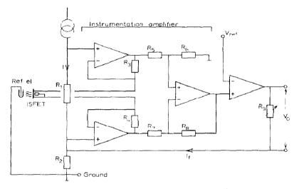
Fig 6 Principle diagram of a source and drain follower
