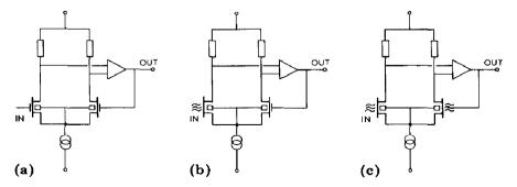
Fig 8 Principle diagrams for differential amplifier circuit with feedback for (a) a pair of MOSFETs, (b) an ISFET and a MOSFET, (c) a pair of ISFETs
