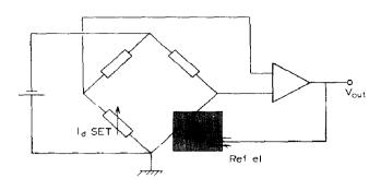
Fig 5 Principle diagram of an automatically balanced bridge circuit
