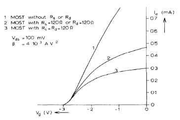
Fig 3  $I_d - V_g$  characteristics of a MOSFET for various values of series resistors in source and drain leads,  $R_s$  and  $R_d$ , respectively 1 MOSFET without  $R_s$  or  $R_d$ , 2 MOSFET with  $R_s = 120 \Omega$  or  $R_d = 120 \Omega$ , 3 MOSFET with  $R_s = R_d = 120 \Omega$ ,  $V_{ds} = 100 \text{ mV}$ ,  $\beta = 4 \times 10^{-3} \text{ A V}^{-2}$
