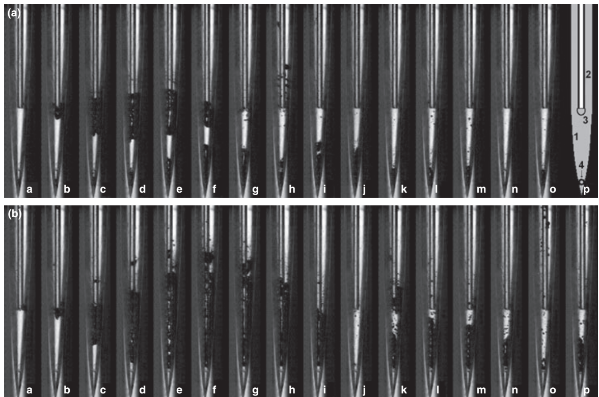
Figure 2 (Video clips S1 and S2) Visualization of the laser-generated vapor bubble. The laser energy was 60 mJ per pulse in (a) and 250 mJ per pulse in (b). Image sequence is from left to right. The interframe time is 140 \mu\text{s} . Panel p in (a) shows a sketch of the setup, with 1) the root canal model, 2) the laser fiber tip (outer diameter 280 \mu\text{m} ), 3) the laser-induced cavitation bubble, and 4) a stable cavitation bubble at the apex.
