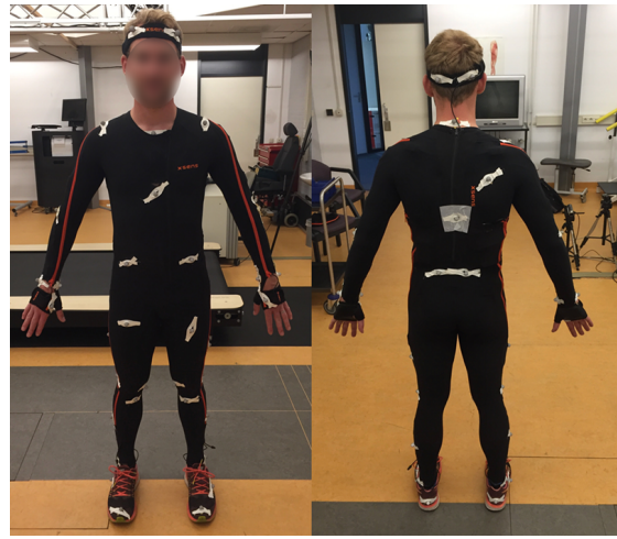
Fig. 1. Placement of the 41 retroreflective markers (according to the Plug-In Gait protocol) 1 can be seen for a representative subject. The markers were placed directly on the subject's skin. IMMU sensors were placed inside a Lycra suit, such that these remain in a fixed position with respect to the body. To accommodate the retroreflective markers, holes were cut in this suit. This allowed for simultaneous measurement of kinematics using optical and IMMU motion capture technologies.
