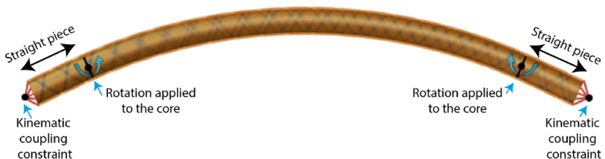
Figure 9. Boundary conditions for the cable bending model.
