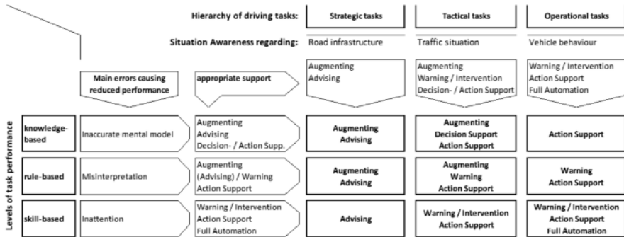
Fig. 3. Assisted driver model showing recommended support types (i.e. levels of automation) dependent on driving situations
