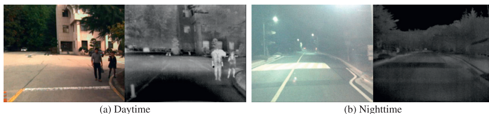
Fig. 7. Samples of false IFCNN prediction results during (a) daytime and (b) nighttime. When the illumination condition is not good during daytime or street lights provide good illumination during the nighttime, the IFCNN model will generate false prediction results.
