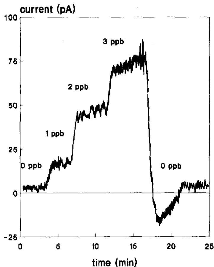
Fig. 6. Sensor response to very small additions of hypochlorous acid showing the sensor's detection limit.
