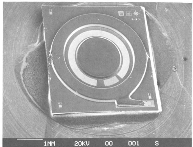
Fig. 3. SEM micrograph of a completed free-chlorine sensor chip.
