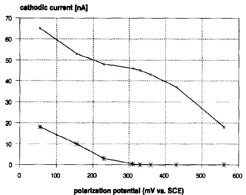
Fig. 4. Cathodic sensor current as a function of polarization potential in phosphate buffer pH 5.5 without chlorine (lower curve) and with 4 mg chlorine/l (upper curve).
