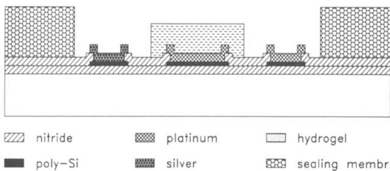
Fig. 2. Cross section of the free-chlorine sensor with electrodes and polymeric membranes.
