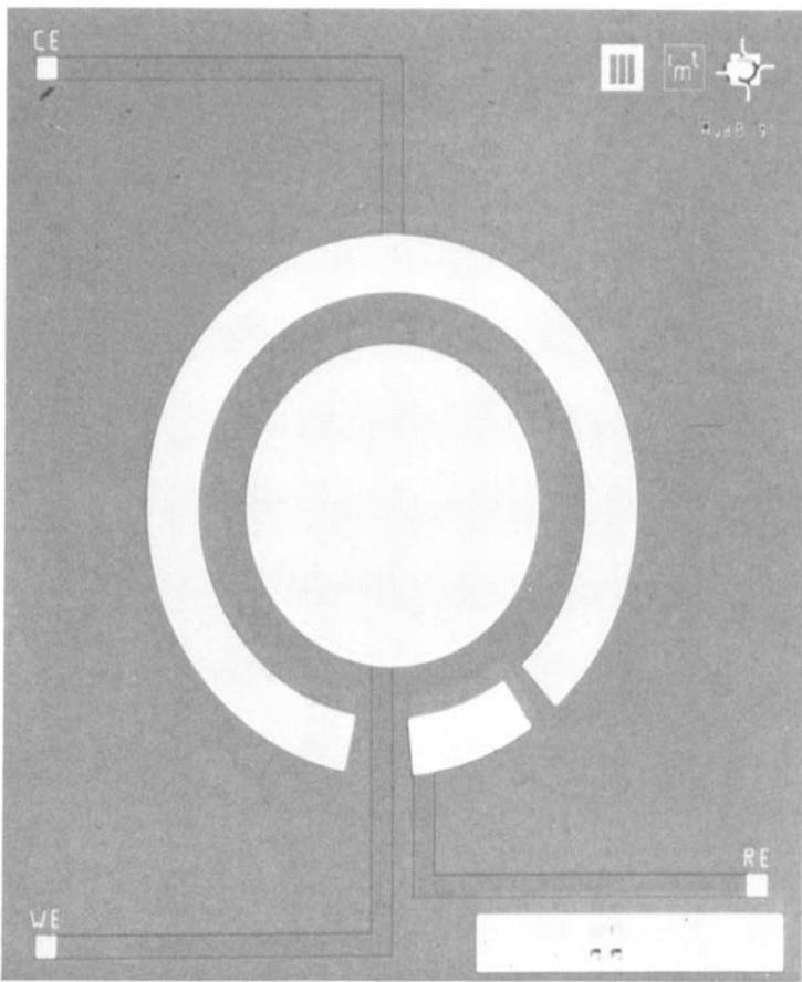
Fig. 1. Photograph of the transducer with platinum working (centre) and counter (ring) electrodes and silver reference electrode (ring-segment) contacted by polysilicon.
