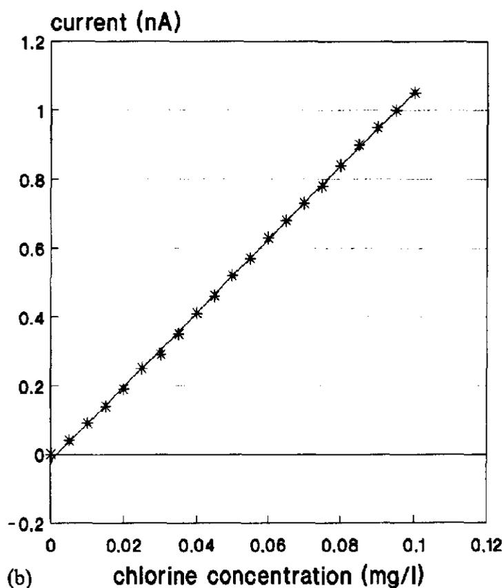
Fig. 5. Sensor output current as a function of hypochlorous acid concentration: (a) high concentration range; (b) low concentration range.
