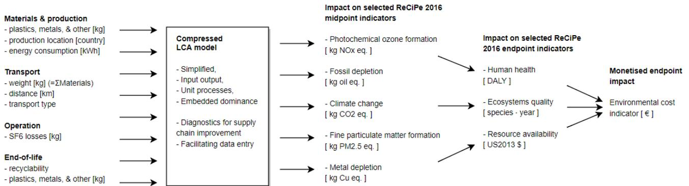
Fig. 4: Image of simplified LCA black box for switchgear - including concrete inputs and outputs
