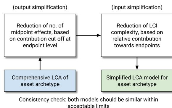
Fig. 1: Conceptual model of LCA simplification process
