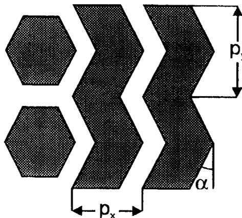
Fig. 2. Schematic layout of the sawtooth shaped biasing strips. The six-angular shapes are the anodes. The parameters  $\alpha$ ,  $p_x$  and  $p_y$  determine the shape.
