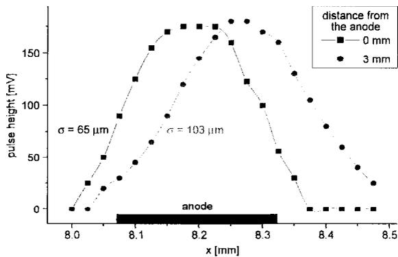
Fig. 3. Charge collection in the small SDD for two distances from the anode. The given standard deviation is that of the assumed gaussian profile of the laser spot including diffusion. The shift of the charge collection area is caused by a rotation of about  $2^\circ$  between the laser and the SDD.
