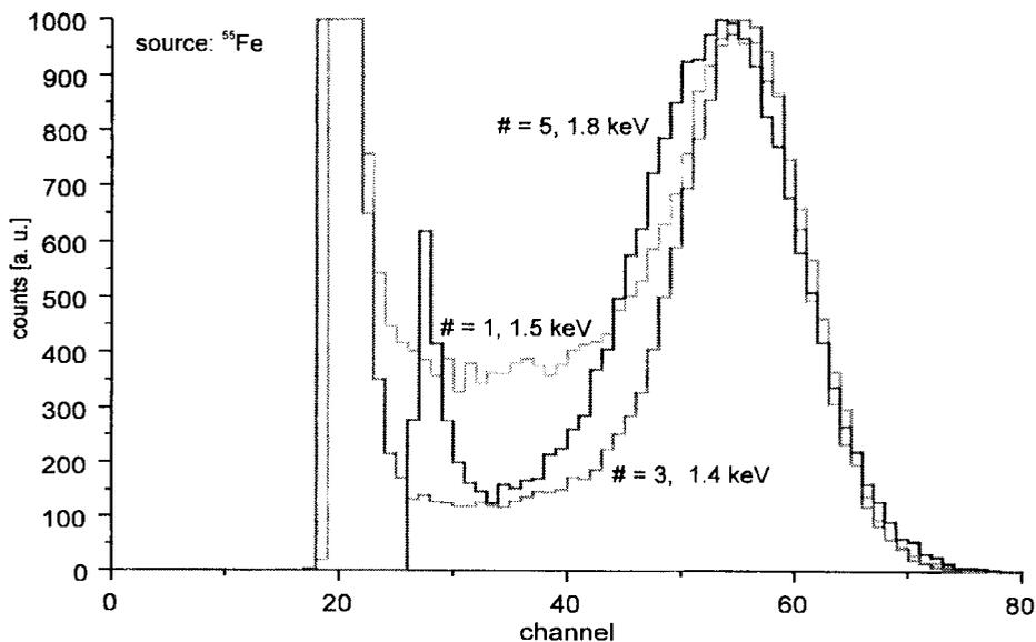
Fig. 4. Energy spectra from a  $^{55}\text{Fe}$  source measured with the small SDD for one, three or five anodes. The FWHM is also indicated in keV.
