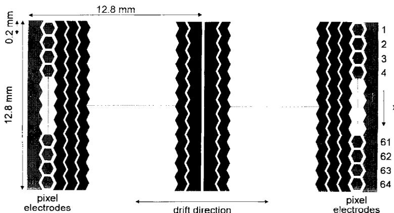
Fig. 1. Schematic layout of the 128 anode drift detector. The sawtooth shape of the biasing strips can diminish lateral diffusion in order to allow spectroscopic measurements.
