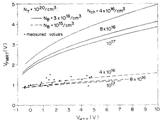
Fig. 9. Simulations of  $V_{FMRT}$  against  $V_{RTT}$  compared to the values measured for the devices represented in Fig. 8.
