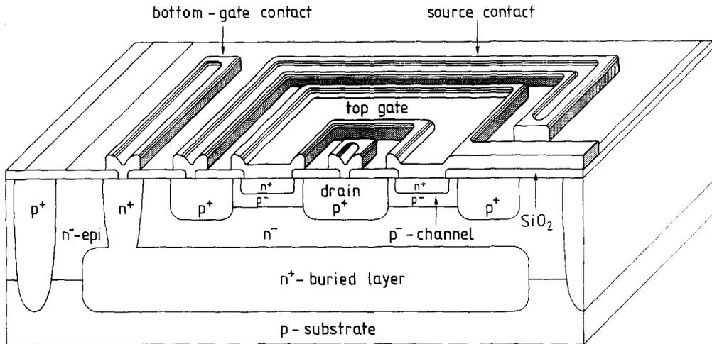
Fig. 1. Basic design of the  $n^+pn^-$  reachthrough diode as it is incorporated in the  $p$ -channel ring-gate JFET, without the second metallization layer.
