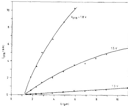
Fig. 13.  $I_{GTB}$  against  $L$  for a set of devices with  $V_{RTT} = 0.7$  V.
