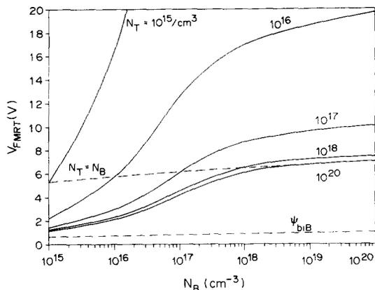
Fig. 7. Simulations of  $V_{FMRT}$  against  $N_B$  for various values of  $N_T$ , with  $N_{ch} = 10^{17}/\text{cm}^2$  and  $V_{RTT} = 5$  V.
