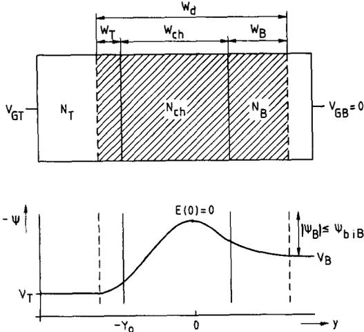
Fig. 3. Nomenclature used to describe the reachthrough diode for  $V_{RTT} \leq V_{GTB} \leq V_{FBT}$ .
