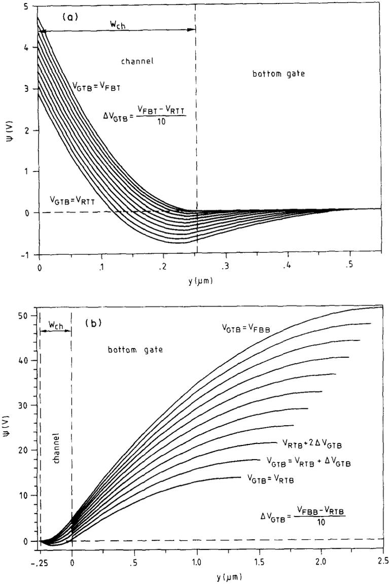
Fig. 4. Simulation of the potential distribution in the depleted region of a  $n^+pn^-$  reachthrough diode as a function of  $V_{GTB}$ , for (a)  $V_{GTB} > 0$ , and (b)  $V_{GTB} < 0$ . The doping levels are  $N_T = 10^{20}/\text{cm}^3$ ,  $N_{ch} = 10^{17}/\text{cm}^3$  and  $N_B = 10^{16}/\text{cm}^3$ , and  $W_{ch} = 0.25 \mu\text{m}$ .
