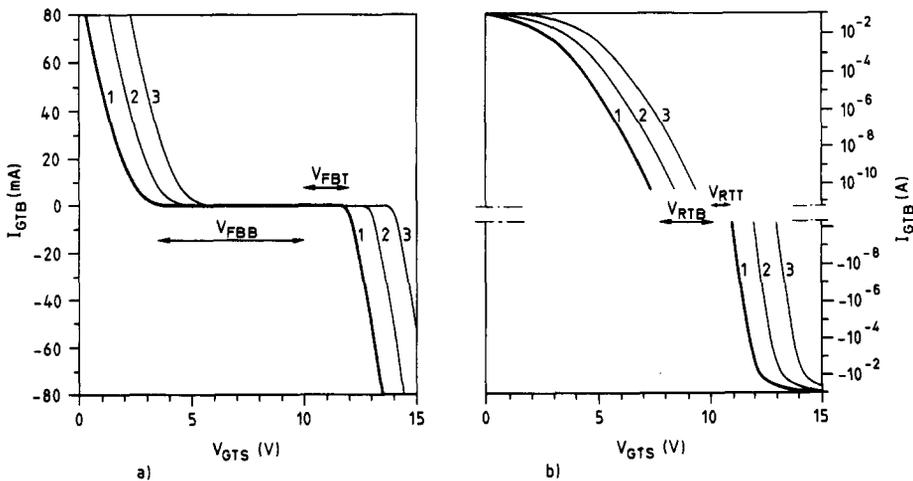
Fig. 6. The linear (a) and logarithmic (b) reachthrough diode characteristics of a device with  $L = 8 \mu\text{m}$ .  $I_{GTB}$  is plotted against  $V_{GTS}$  with  $V_{GBS}$  fixed at (1) 10 V, (2) 11 V and (3) 12 V. The reachthrough and flatband voltages are indicated for the bold curve (1).
