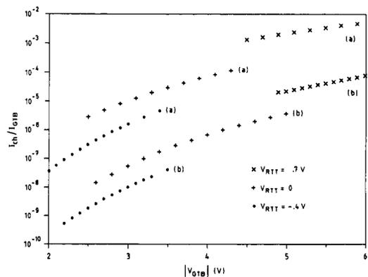
Fig. 12. The ratio of  $I_{ch}$  to  $I_{GTB}$  against  $V_{GTB}$  for three devices with  $L = 2 \mu\text{m}$ , for (a)  $V_{GTB} > 0$ , and (b)  $V_{GTB} < 0$ .
