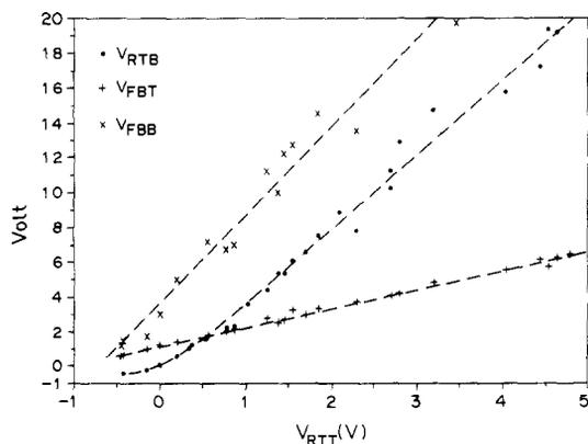
Fig. 8. Experimentally determined relationship between  $V_{RTT}$ ,  $V_{RTB}$ ,  $V_{FBT}$  and  $V_{FBB}$ , for a variety of devices produced with a channel implantation energy between 40 and 150 keV, and a dose between 0.5 and  $12.5 \times 10^{13}/\text{cm}^2$ .
