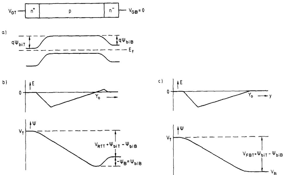
Fig. 2. Schematic illustration of (a) the energy band of a  $n^+pn^-$  structure at thermal equilibrium, and (b) the electric field and potential distributions at the reachthrough condition and (c) at the flatband condition.
