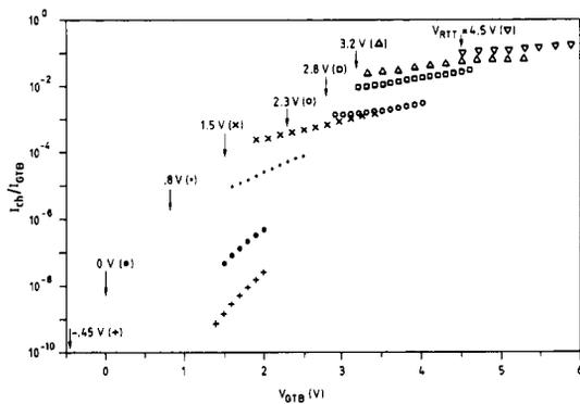
Fig. 11. The ratio of  $I_{ch}$  to  $I_{GTB}$  against  $V_{GTB}$  for devices with  $L = 2 \mu\text{m}$ . The interval between reachthrough and the onset of measurable  $I_{ch}$  is visualized by an arrow indicating  $V_{RTT}$ .
