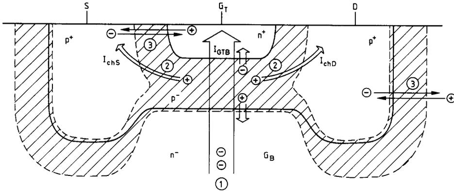
Fig. 10. Currents in a JFET structure with  $V_{DS} = 0$  and the reachthrough diode biasing  $V_{GTB} > V_{RTT}$ . The depleted regions are shaded and the indicated currents are (1)  $I_{GTB}$ , (2) Impact-ionization currents, and (3) diode leakage currents.
