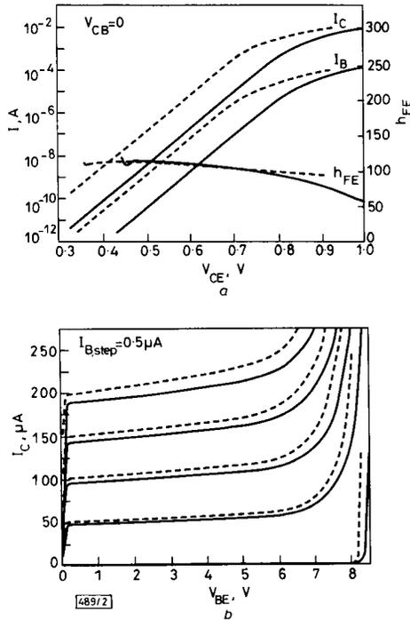
Fig. 2 Gummel plots and output characteristics of two 15 GHz WEB NPNs, with  $A_E = 20 \times 1 \mu\text{m}^2$  or  $20 \times 40 \mu\text{m}^2$
