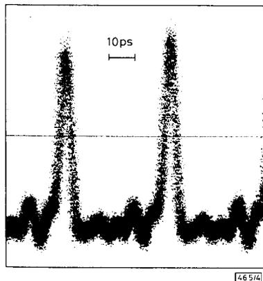
Fig. 4 Experimentally generated pulse trains at 5 GHz repetition rate
