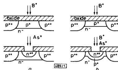
Fig. 1 Schematic presentation of a conventional washed-emitter NPN implantation scheme and the WEB implantation scheme
