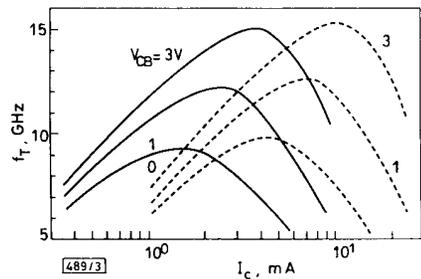
Fig. 3 Cutoff frequency against collector current for two 15 GHz WEB NPNs, with  $A_E = 20 \times 1 \mu\text{m}^2$  or  $20 \times 4 \mu\text{m}^2$
