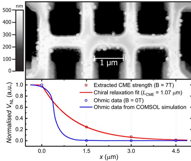
FIG. 5. Diffusion lengths. Top: Atomic force microscopy image of a Bi<sub>0.97</sub>Sb<sub>0.03</sub> single-crystal flake, structured into a device for nonlocal measurements and contacted with Nb leads. Bottom: Normalized strength of the Ohmic (zero field) and CME (from fit) contributions to the signals measured at the voltage probes. The CME strength persists over longer distances than the Ohmic signal.
