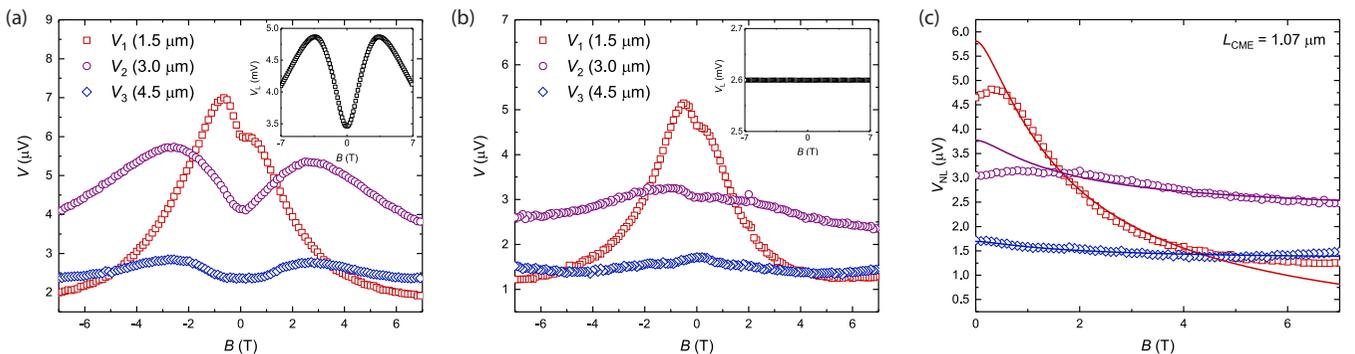
FIG. 4. Nonlocal signals. (a) Measured voltages at distances 1.5, 3 and 4.5  $\mu\text{m}$ . The inset shows the local voltage, measured at the source contacts. (b) Same as in (a), but for a varying source current  $I_s(B)$  such that  $V_L = \text{cst.}$  (inset). (c) Symmetrized nonlocal voltages for fixed local electric field,  $V_{NL}(E = \text{cst.}, B)$ , from (b).
