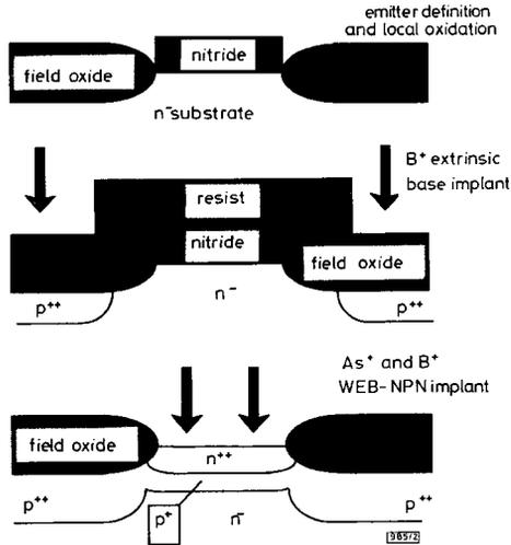
Fig. 2 Basic WEB NPN process flow with LOCOS isolated emitter
