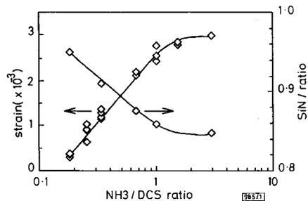
Fig. 1 Film strain and ratio of silicon to nitrogen in film against  $\text{NH}_3/\text{DCS}$  gas flow ratio
