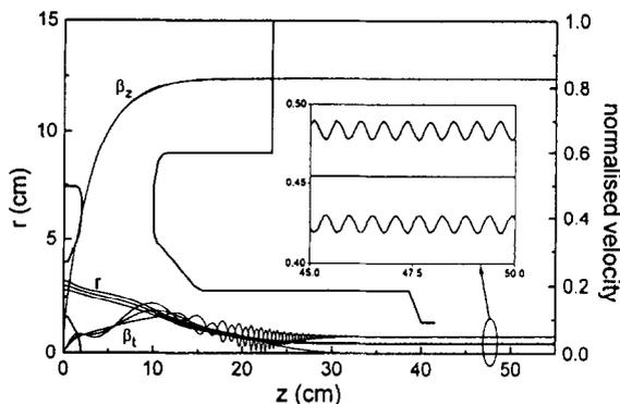
Fig. 1. Electrode configuration and electron trajectories.
