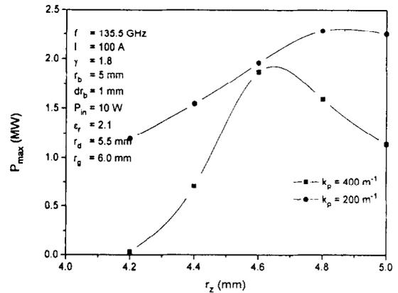
Fig. 3. Maximum power as a function of  $r_z$ .
