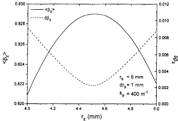
Fig. 2. Average velocity and spread as a function of  $r_z$ .
