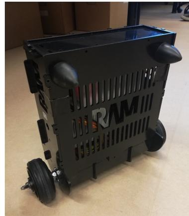
Fig. 5. The mini-segway used in this example, motor drivers, and Inertial measurement unit (IMU) and absolute wheel encoders.
