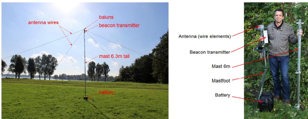
Figure 1: (left) The beacon transmitter is mounted at the feed point of the wire dipoles, and is fed from a 13.5 Volt battery located at the foot of the mast. (right) The entire system is easily transported and can be set-up by a single person in 1.5 hours.
