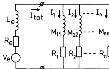
Fig. 1. Equivalent circuit of the n-strand cable.
