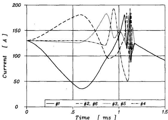
Fig. 6. Simulated quench process for a 6-strand cable.
