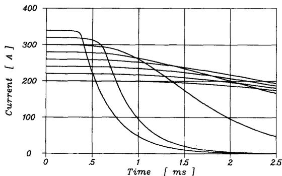
Fig. 5. Decay of the total current of a 2-strand cable for different starting currents.
