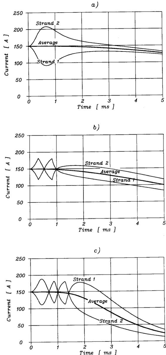
Fig. 3. Examples of different assumptions in the model: a) one normal spot starting with  $R=0$ , b) appearance of step-resistances  $\Delta R$ , c) several spots, i.e. propagation at  $v_p=mI$ .
