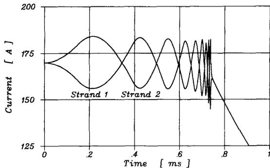
Fig. 4. Calculated fast quench for  $I(0)=170$  A/strand.
