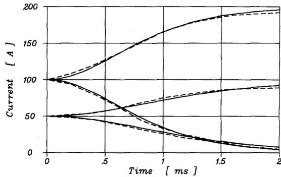
Fig. 2. Calculated (—) and measured (---) redistribution of current in a 2-strand cable.
