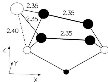
FIG. 3. Perspective view of the equilibrium binding configuration showing the first-, second-, and third-layer substrate atoms as in Fig. 1, and the bond lengths in angstroms. The adatom is shown as a large open circle.
