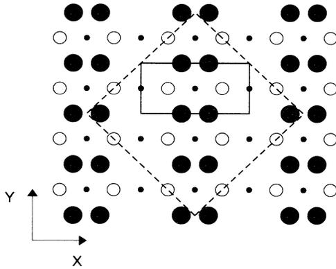
FIG. 1. Projection of the topmost three layers of the  $p(2 \times 1)$ -reconstructed Si(100) surface. The large solid circles represent the top-layer atoms, the medium-sized open circles represent the second-layer atoms, and the small solid circles represent the third-layer atoms. The  $p(2 \times 1)$  unit cell is indicated by the solid line and the  $p(\sqrt{8} \times \sqrt{8})R45^\circ$  unit cell (Ref. 10) by the dashed line.
