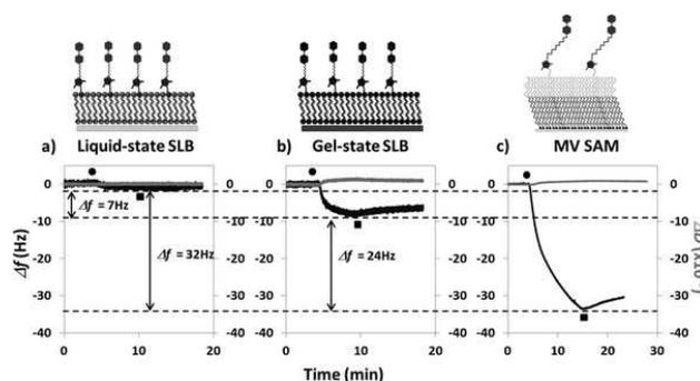
**Figure 1.** QCM-D response plots to flowing  $1 \times 10^{-6}$  M ConA (●) over a) a liquid-state SLB, b) a gel-state SLB, and c) an oligoethyleneglycol-based SAM, each with 1% surface density of MV followed by rinsing with buffer (■). Change in frequency ( $\Delta f$ , black) and dissipation ( $\Delta D$ , gray) values correspond to the fifth overtone.
