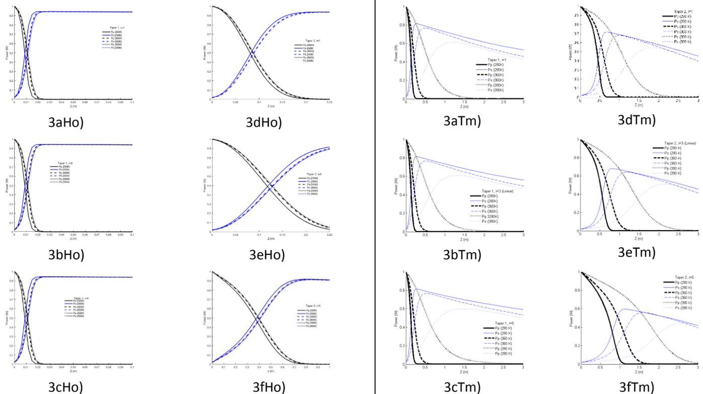
**Fig. 2** Evolution of pump and signal radiations at different temperatures for Ho and Tm fibers
