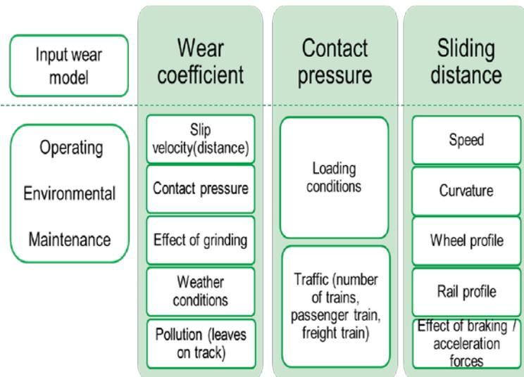
Figure 4: Coupling between usage parameters and input parameters of the wear model.
