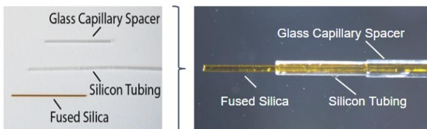
**Figure S2. Exchangeable nozzle assembly.** To assemble an exchangeable nozzle, a fused silica capillary was inserted into a silicone tubing, which was inserted into a glass capillary spacer.
