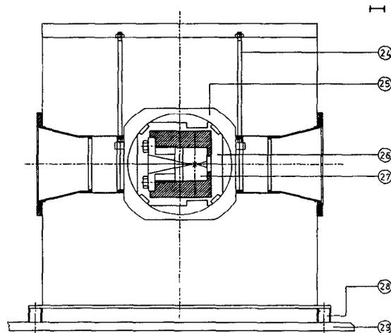
FIG. 2. Cross section through the plane that is parallel to the optical axis and parallel to the vertical axis of the cell. The bar (top right) indicates a length of 1 cm. The numbers denote the following components. 24: rod; 25: main cylinder; 26: spacer; 27: diamond-anvil cell; 28: spacer; 29: plate.
