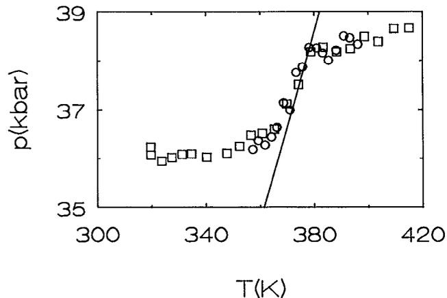
FIG. 5. Quasi-isochoric  $p$ - $T$  scan through the melting line of pure nitrogen. Different symbols indicated different scans. The drawn line is the smoothed melting curve of Ref. 11.
