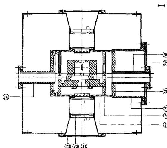
FIG. 3. Cross section of the HTDAC through the horizontal plane, parallel to the optical axis of the thermostat. The bar (top right) indicates a length of 1 cm. The numbers denote the following components. 25: main cylinder; 26: spacer; 27: glass cylinder; 28: cover; 29: cover; 30: glass cylinder; 31: quartz window; 32: quartz window; 33: quartz window; 34: glass cylinder.
