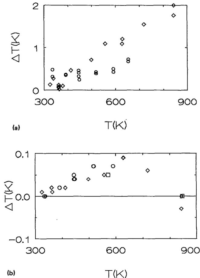
FIG. 4. (a) Temperature between the diamonds minus temperature below the bed (vs temperature between the diamonds). (b) Temperature between the diamonds minus temperature on ring No. 12 vs temperature. In all graphs, circles indicate run 1, diamonds run 2, and squares run 3.
