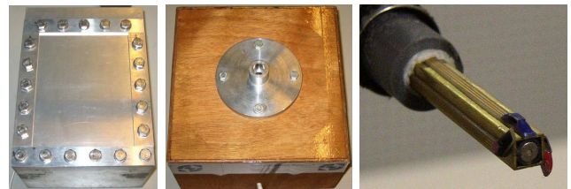
Figure 2: aluminium box, incoming noise source and sensor
