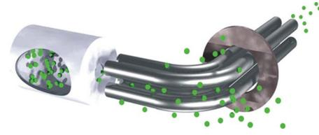
FIG. 2. (Color online) Schematic of the experiment. On the left is the effusive source, which injects thermal  $D_2O$  molecules into the four-wire guide. Neighboring electrodes have opposite polarity, creating a quadrupolar electric field. Molecules that are slow enough are guided through the first and second (not shown)  $90^\circ$  bends and are finally detected by a mass spectrometer.
