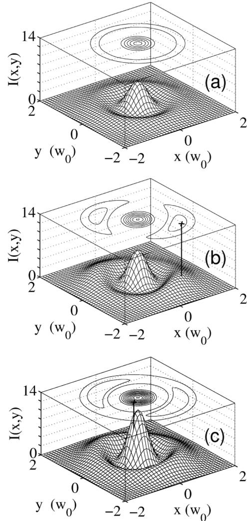
FIG. 1. Transversal spatial intensity pattern of the stationary cavity field for the empty cavity (a) and two atomic positions indicated by the thick vertical line and a cross (b), (c).
