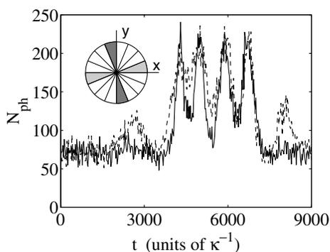
FIG. 3. Simulated photon flux (number of photons  $N_{\text{ph}}$  per 100  $\kappa^{-1}$ ) measured at two out of 8 photodetector pairs as a function of time (units of  $\kappa^{-1}$ ). The inset depicts the arrangement of the detectors on the cavity output, shaded areas correspond to the plotted curves.
