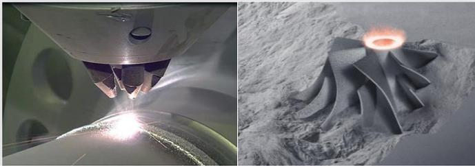
Figure 1: Directed energy deposition [1] (a), Powder bed fusion [2] (b)
