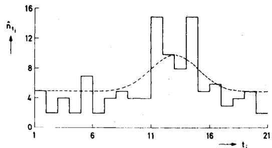
Fig. 5. Simulated Poissonian pulse train (drawn line) and  $\lambda_{t_i}$  of (30) (dotted line), with parameter setting  $\alpha = 2.0$ ,  $a = 13.0$ ,  $\lambda_0 = 3.0$ ,  $\beta = 2.5$ ,  $s = 2.0$ ,  $m = 21$ .
