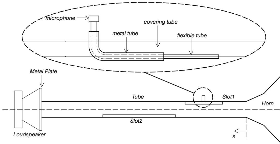
Fig. 3: Measurement set-up according to Fahy's method, with magnified microphone-probe set-up. Measuring microphone can be inserted in one of both slots.
