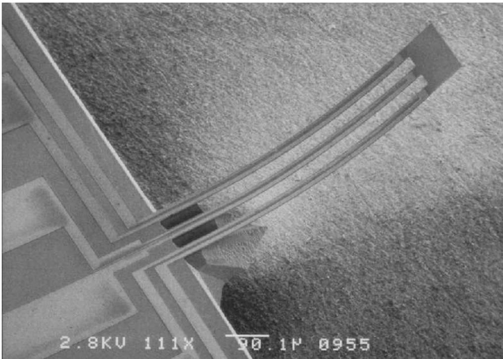
Fig. 4: The  $\mu$ -flown, showing the three cantilever shaped resistors of which the outer two are used as sensing resistors while the middle resistor is used as heater.
