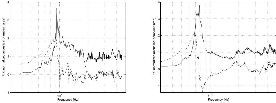
Fig. 5: Measurement results of Fahy's (left hand-side) and direct (right hand-side) method. Solid lines depict normalized throat resistance  $R$  and dashed lines normalized throat reactance  $X$ .
