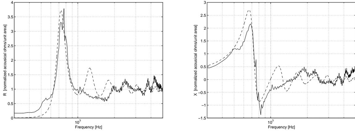
*Fig. 8: Optimized simulation results of the hyperbolic horn approximation with 10 conical elements (dashed lines) on measurement results of direct method (solid-lines). Left hand-side shows normalized throat resistance  $R$  and right hand-side normalized throat reactance  $X$ .*
