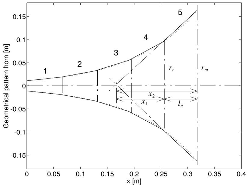
Fig. 2: Modeling of a horn by 5 equal length ( $l_c$ ) conical elements. Distances to apex for final element are shown.
