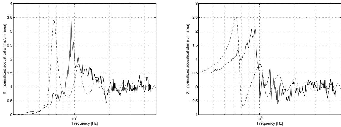
Fig. 6: Measurement results of Fahy's method (solid-lines) compared with simulation results of hyperbolic horn approximation with 10 conical elements (dashed lines). Left hand-side shows normalized throat resistance  $R$  and right hand-side normalized throat reactance  $X$ .
