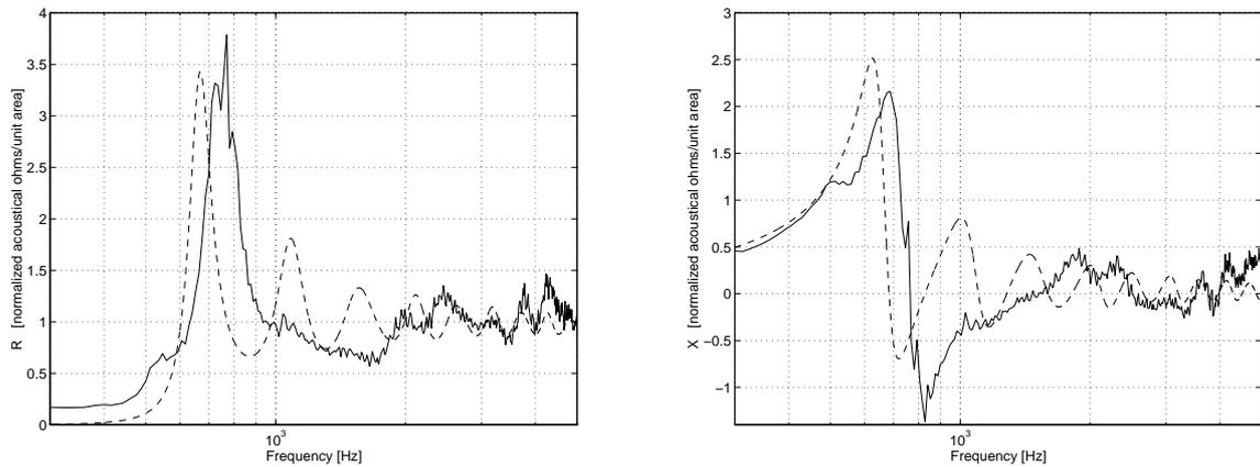
Fig. 7: Measurement results of direct method (solid-lines) compared with simulation results of the hyperbolic horn approximation with 10 conical elements (dashed lines). Left hand-side shows normalized throat resistance  $R$  and right hand-side normalized throat reactance  $X$ .
