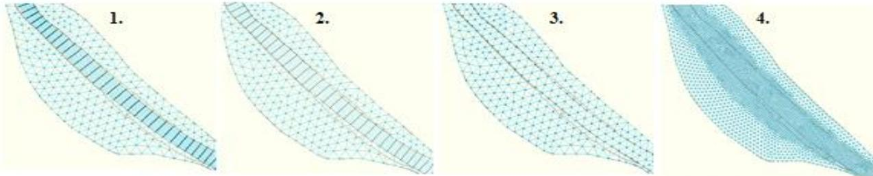
Figure 1: The four grid types studied, in which grid 1 and 2 represent the hybrid grid types and grid 3 and 4 the complete triangular grids.
