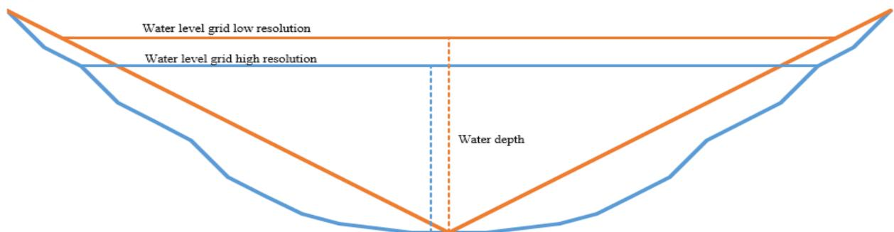
Figure 2: Example of discretization of the summer bed geometry for a grid with only two grid cells in the summer bed (orange) and a grid with a much finer resolution (blue).
