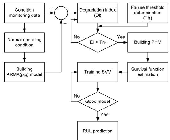
Fig. 13 Schematic diagram of proposed method
