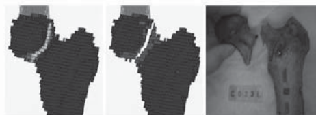
Fig2: Failure location in FE-model and experiment
