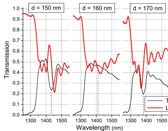
Fig. 3. Calculated Transmission ( $T$ ) and Loss ( $L$ ) spectra (obtained as  $L = 1 - (T + R)$ ,  $R$  standing for Reflectance) relevant to three geometrical configurations. For recess depth  $d = 160$  nm, the stop-band disappears. Note the opposite slope of the loss curve within the stop-band region for  $d = 150$  nm and  $d = 170$  nm. The gratings are 16-periods long.
