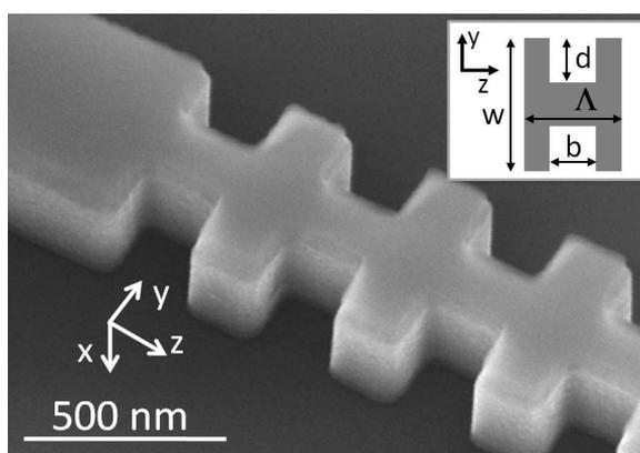
Fig. 1. Scanning electron micrograph giving a 'bird's-eye' view of photonic wire Bragg grating fully etched into silicon waveguide core layer. Inset: top view, defining dimensions.
