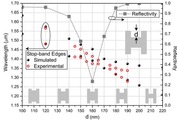
Fig. 4. Positions of numerical (black filled circles) and experimental (red empty circles) transmission stop-band of PhWBG in dependence on the recess depth  $d$ . The reduction of stop bandwidth is consistent the reduction of numerical maximum reflectance (crossed diamonds)
