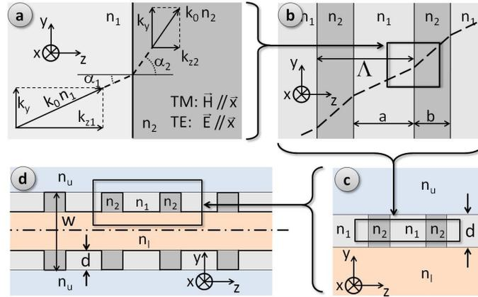
Fig. 5. Sketch of the steps of the theoretical model. (a) Semi-infinite interface. (b) 1D-stack grating. (c) Laterally confined 2D grating. (d) Photonic Wire Bragg Grating.
